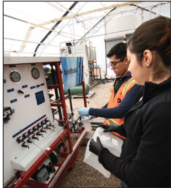
Taking samples from the nanofiltration process at the Advanced Water Purification Pilot Facility.
