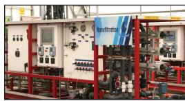
In the next step, water is forced under high pressure through non-porous semi-permeable membranes that remove dissolved salts. metals, dissolved organic molecules and other materials, many of which are more than 50,000 times smaller than the smallest bacteria or virus. This is the same process used by some bottled water companies, baby food manufacturers and for kidney dialysis.
