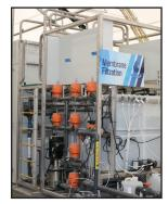
Two types of membrane filtration are being tested – microfiltration and ultrafiltration – to determine which is most effective for a full-scale plant. In this initial filtration stage, water is
