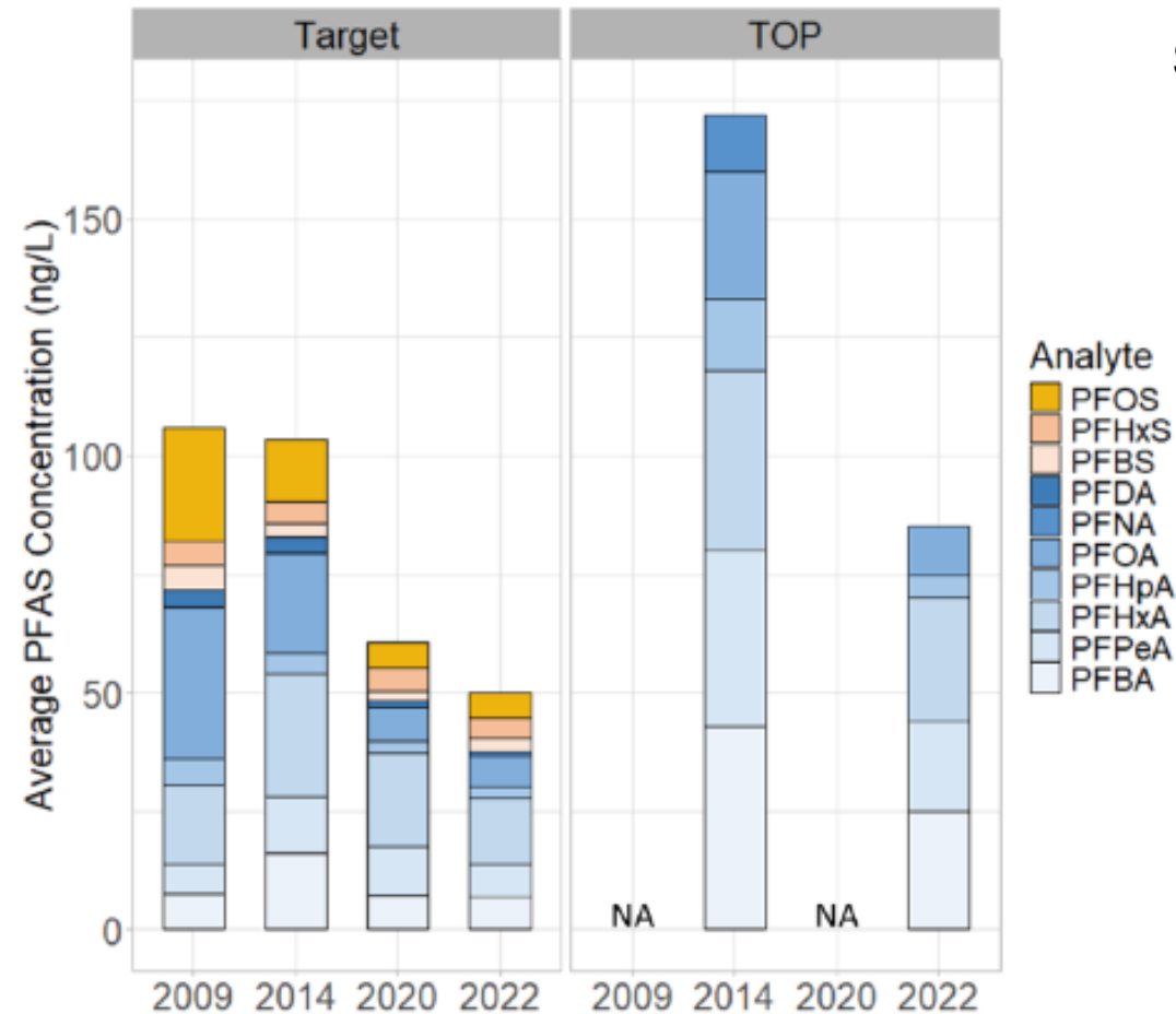
Figure 3.3: Average concentration of detected PFAS in San Francisco Bay POTW final effluent. The TOP assay was not applied for samples from 2009 and 2020.
