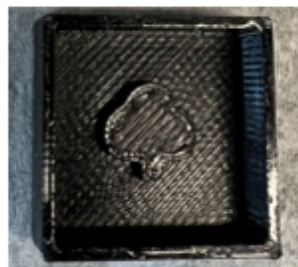
3D printed plastic mold
