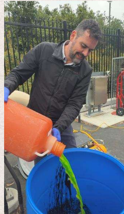
Preparing the Fluorescein dye (fluorescent dye tracer used)
