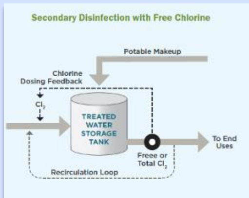
FIGURE 8.4: Secondary disinfection with free chlorine [SFPUC Onsite Water Reuse Program Guidebook p28 Graphics]
