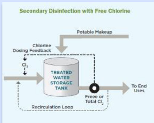
FIGURE 8.4: Secondary disinfection with free chlorine [SFPUC Onsite Water Reuse Program Guidebook p28 graphics]
