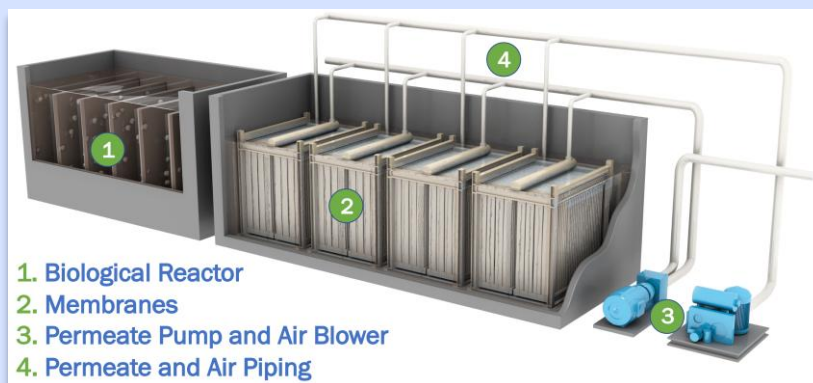
FIGURE 6.2: Schematic of an MBR [NBRC ONWS Guidance Manual p33 Figure13]
