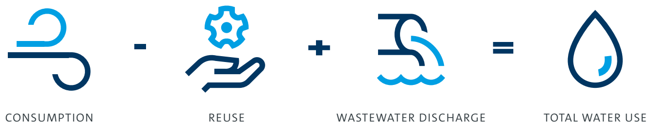
Figure 5: The water balance approach. Consumption plus discharge minus reuse equals the water use. The water balance is then used for the process balance utilizing assumption of the water usage for the different processes: boiler water, cooling water, process water and other purposes.
