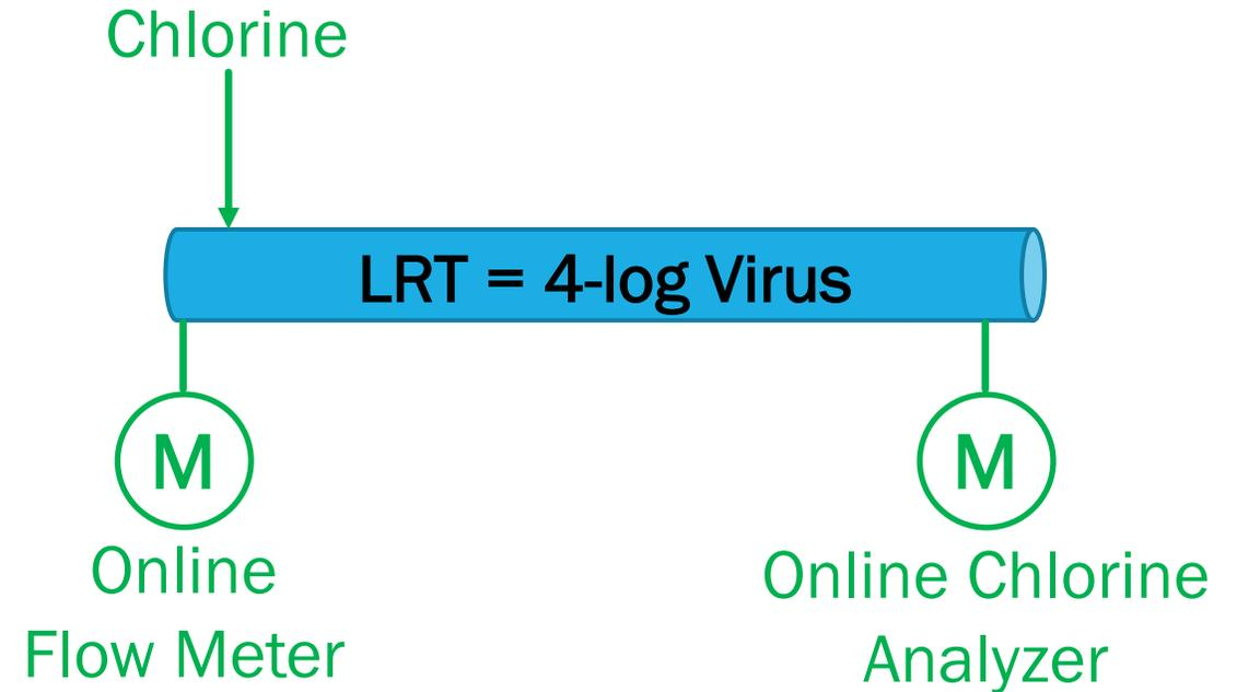
Online verification of chlorine residual and flow rate confirms LRV continuously
