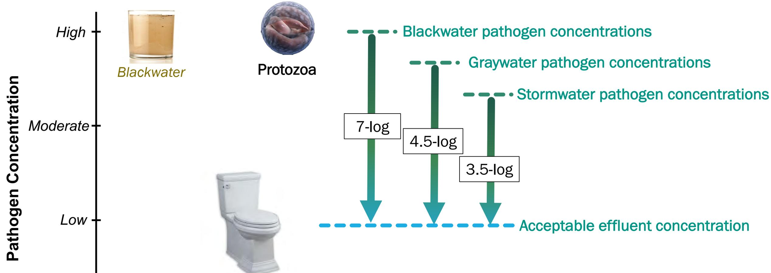
The LRTs are designed to produce non-potable water that meets the same risk-based goal for all types of source waters
