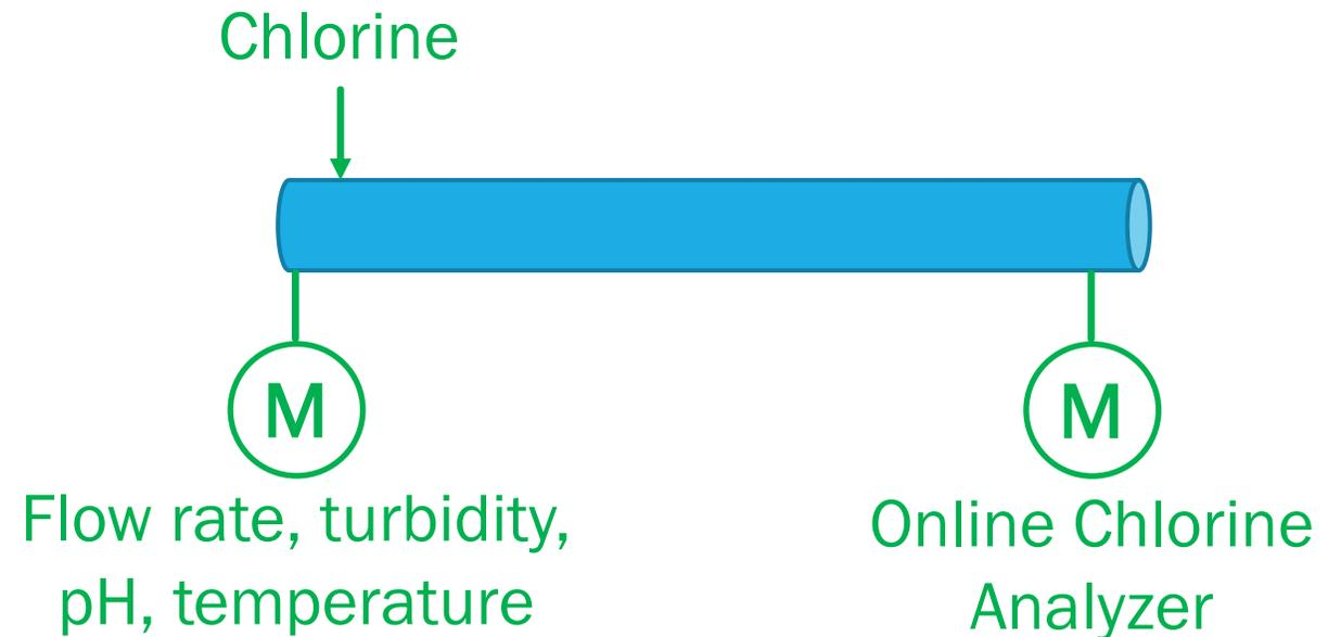
Continuous verification of chlorine residual and flow rate confirms LRV continuously
