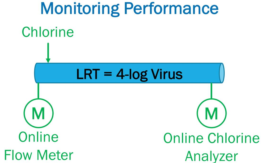
Online verification of chlorine residual and flow rate confirms LRV continuously
