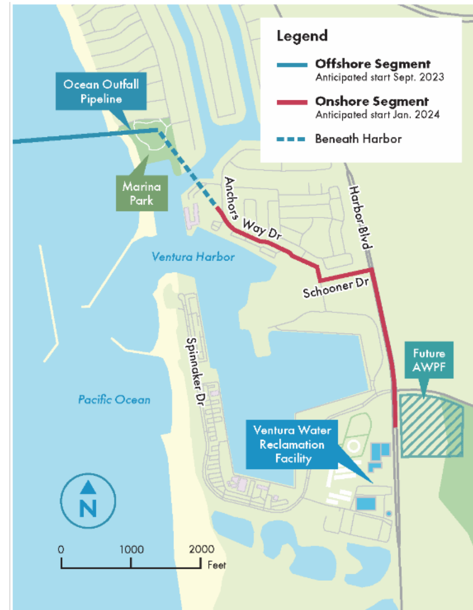
Typical ROC disposal – Ventura Water Pure
