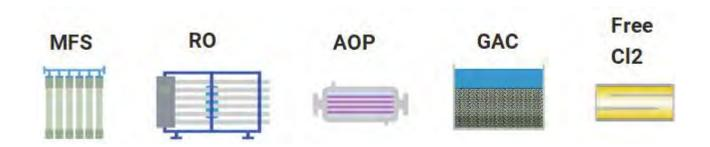
Piping and control system will have flexibility to operate GAC Before UVAOP A small chiller and calcite contactor will be added at the end for water testing
