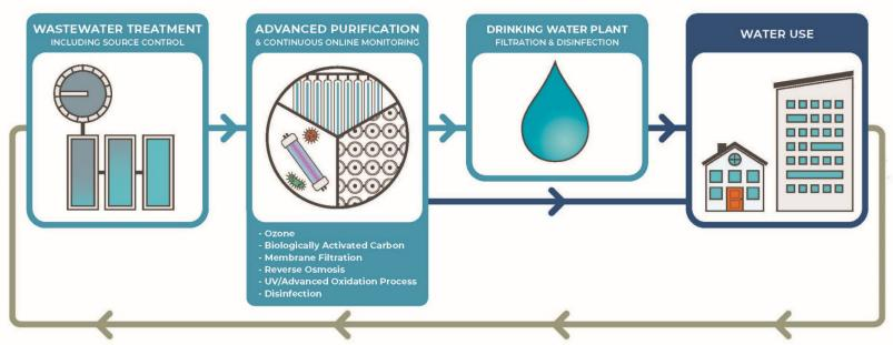
Direct Potable Reuse treatment steps described by Cailfornia regulations announced in Dec 2023. Final purified water meets all drinking water standards and stringent regulations for emerging contaminants.
