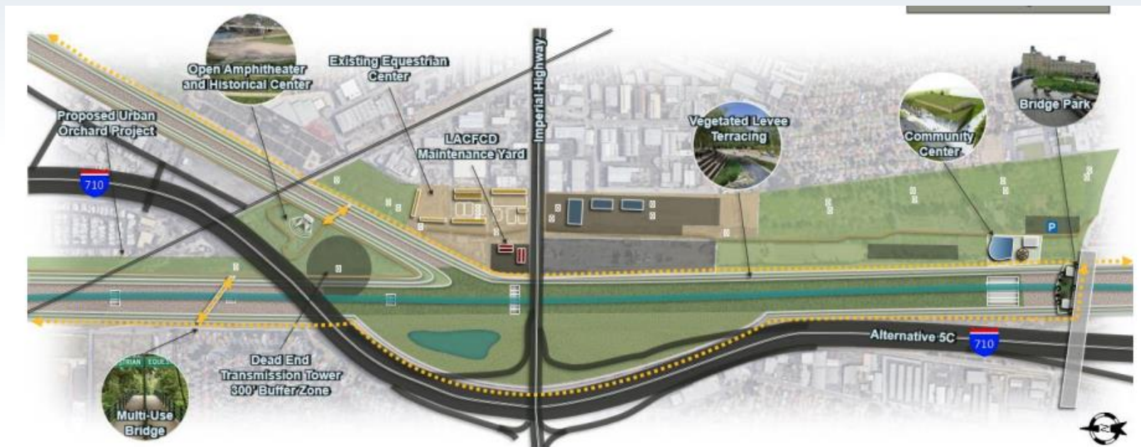
Figure 3.4-10. Configuration 3 Conceptual Layout – Soft-Bottom River with Relief Drain
