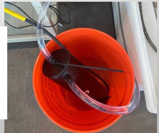
Turner Cyclops C3 Submersible Sensor
