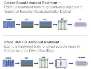
Chart 1: EXAMPLES OF OZONE/BAC TREATMENT TRAINS FOR POTABLE REUSE
