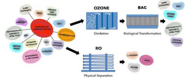
Chart 2: SOURCE WATER INPUT AND REMOVAL OF CECs WITH OZONE/BAC AND RO
