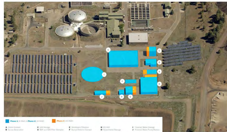
Figure 2-6. O 3 /BAF-Based Treatment at Wildcat Hill
