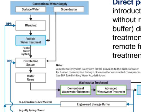
**Direct potable reuse (DPR):** The introduction of reclaimed water (with or without retention in an engineered storage buffer) directly into a drinking water treatment plant, either collocated or remote from the advanced wastewater treatment system.
