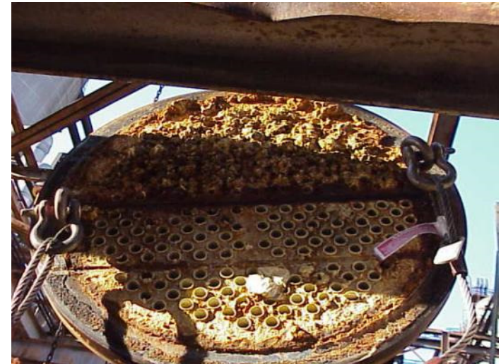
Heat exchanger tube sheet: Heavy mineral and bio deposits
