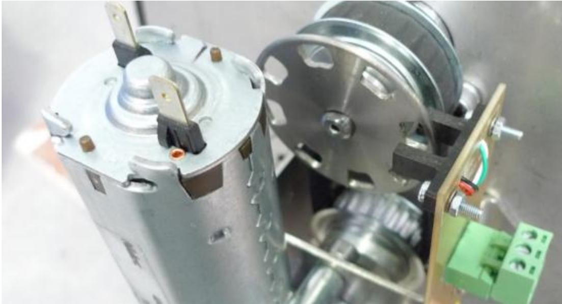
Optical counter used to stop wiping mechanism before reaching the chamber ends. Similar technology used in elevators to signal floor levels. No problematic limit switches are required.
