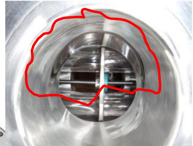
The profile of the hatch was designed to eliminate flow disruptions and air pockets.
