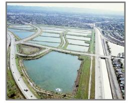
Aquifer Injection / Spreading
