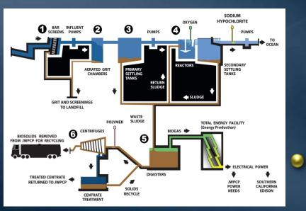
Design flow rate 400 MGD; current flow rate 265 MGD
