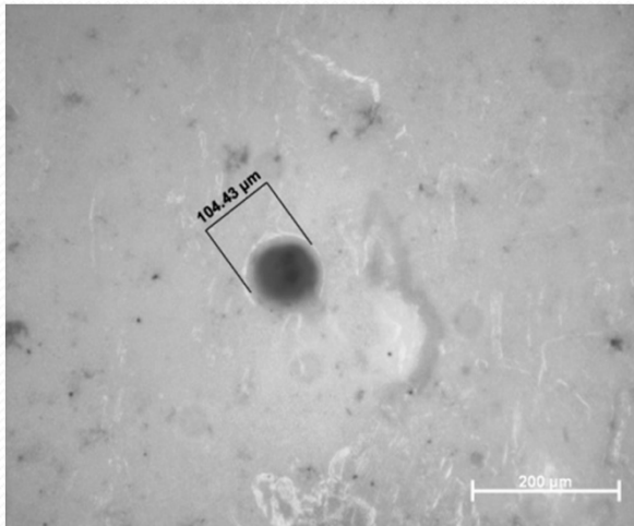
Large pinhole No. 1: 104 µm diameter
