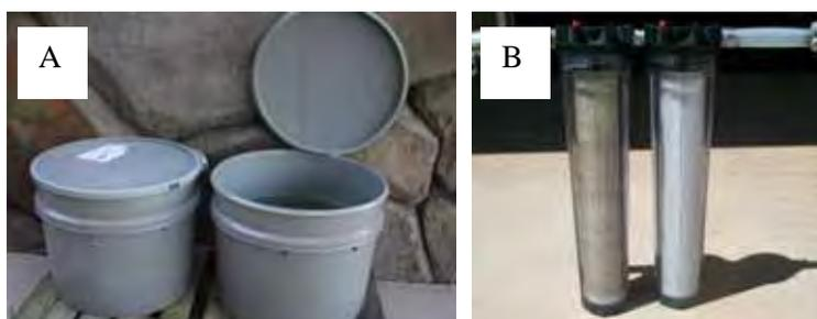
**Figure 2.1. Wastewater collection containers and laboratory filtration apparatus.**
