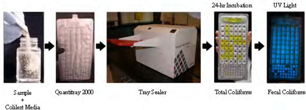
**Figure 2.5. Colilert method for total and fecal coliforms.**
