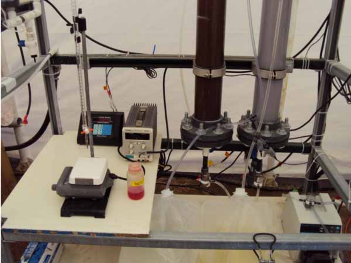
Figure 6.3. Pilot equipment including timer (far left), power supply (middle), titration setup (front), and regeneration pump (far right).
