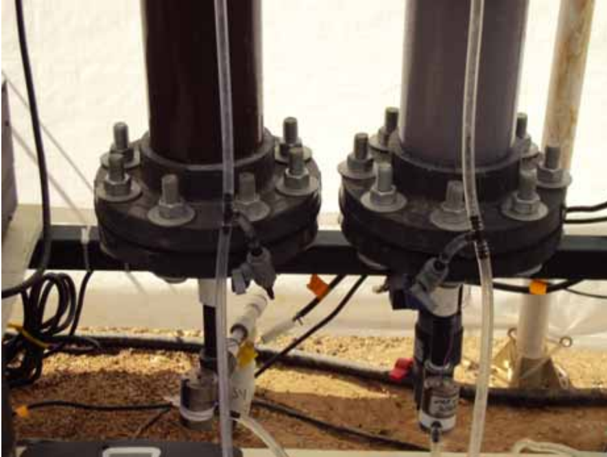
Figure 6.5. Solenoid valves at bottoms of columns.
