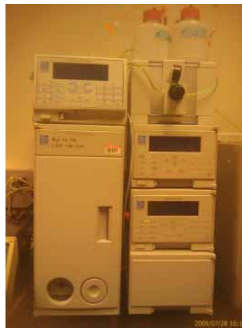
Figure 3.2. Atomic absorption spectrometer (left) and ion chromatography system (right).
