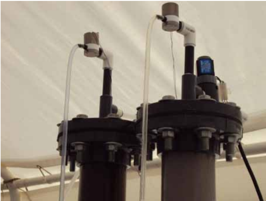
Figure 6.4. Solenoid valves at tops of columns.
