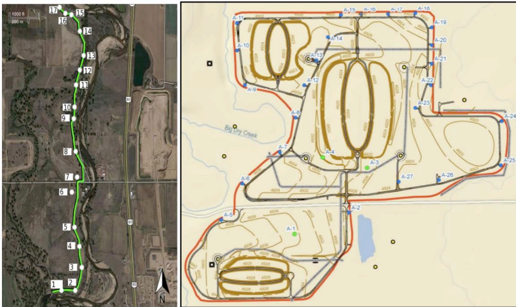
Figure 2.1. Aerial map of the RBF well field along South Platte River at Brighton and map of the adjacent aquifer recharge and recovery site including well locations.
