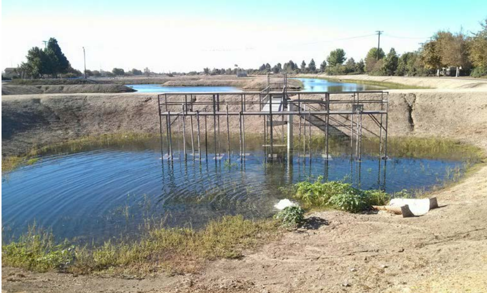
Figure 2.5. Montebello Forebay test basin during wetting operation for microbial community activation (November 5, 2012).
