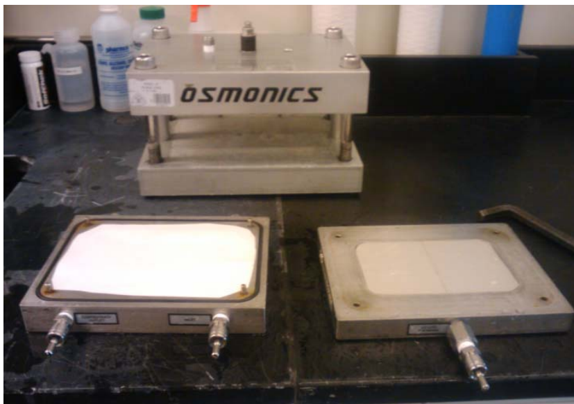
Figure 3.4. SEPA II membrane testing unit employing flat-sheet membrane.
