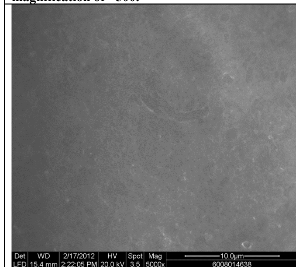
Figure D.8.5. ESEM micrograph of thin biofilm at magnification of ×5000.
