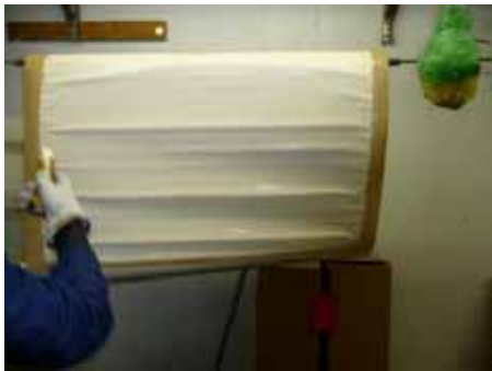
Figure 5.18. Photographs illustrating the process of sampling RO elements for microscopy analysis.
