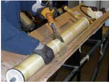
Figure 5.17. Photographs illustrating the process of opening the RO elements.
