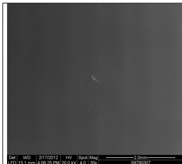
Figure D.4.1. ESEM micrograph of MBR-O 3 -RO lead element at magnification of ×30. Membrane surface was quite clean, similar to virgin membrane.
