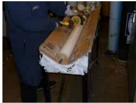
Figure 5.17. Photographs illustrating the process of opening the RO elements.
