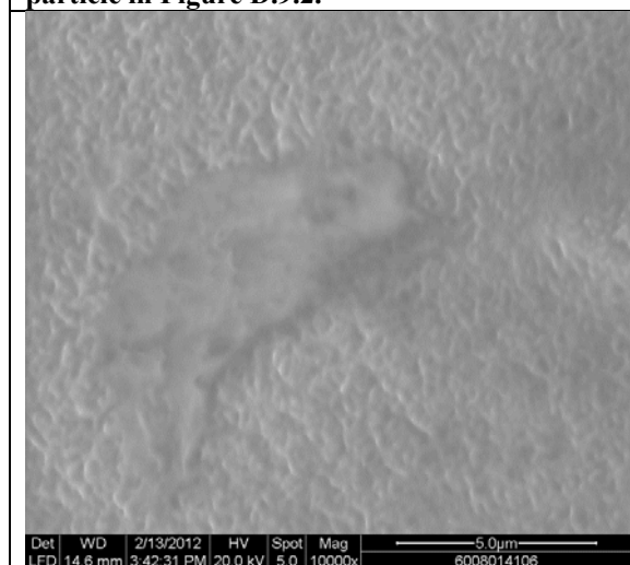
Figure D.9.5. ESEM micrograph of biofilm formation at magnification of \times 10,000 .
