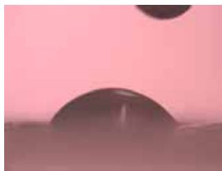
Figure 2.2. Image from sessile drop method using water on a fouled membrane surface.
