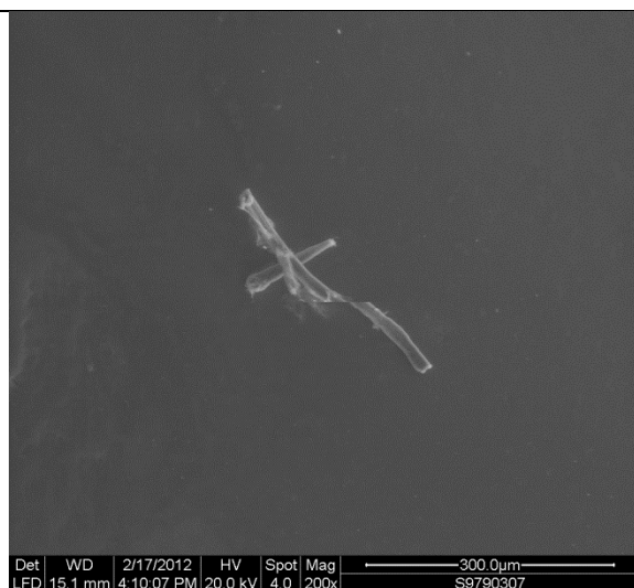
Figure D.4.2. ESEM micrograph of broken hollow-fiber membrane pieces at magnification of ×200.
