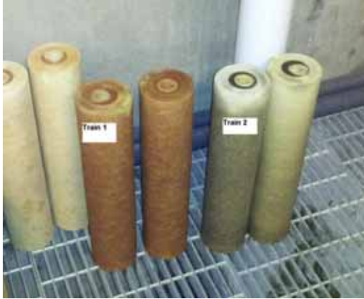
Figure 6.10. Photograph of cartridge filters from UF-UV/H 2 O 2 -RO (Train 1) and UF-RO (Train 2) trains under 14-gfd conditions.
