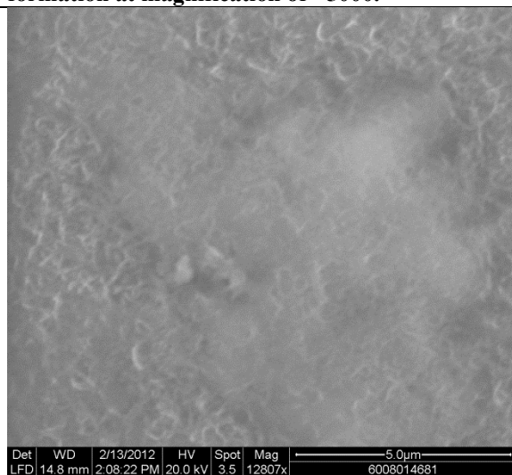
Figure D.6.6. ESEM micrograph of biofilm formation at magnification of \times 13,000 .
