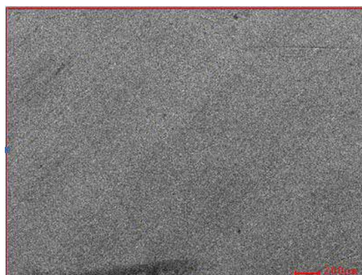
Figure 5.22. SEM image at ×40 (the scale bar in red is for 200 μm) of a sample of MBR-O 3 -RO tail element (left image) and a table generated from EDAX analysis.
