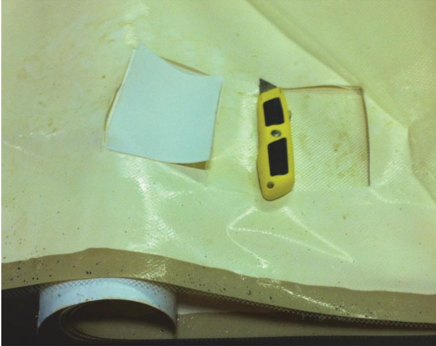
**Figure 6.13. An example of the size of the membrane specimens and their location relative to the edge of the RO elements.**
