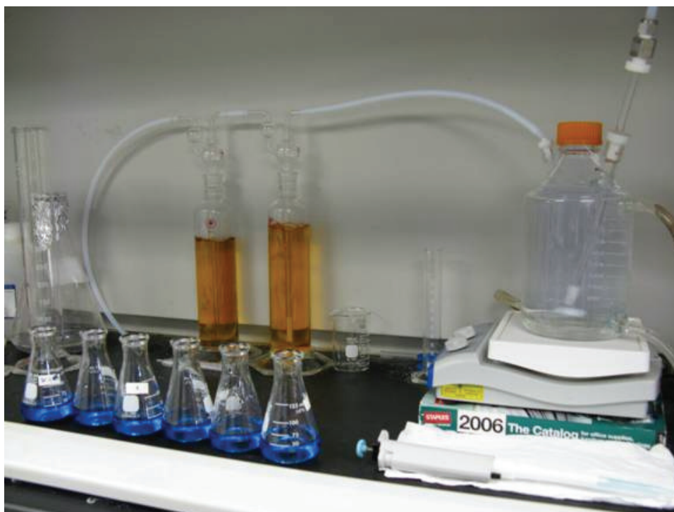
Figure 2.2. Equipment used to generate O_3 stock solution in batch mode.
