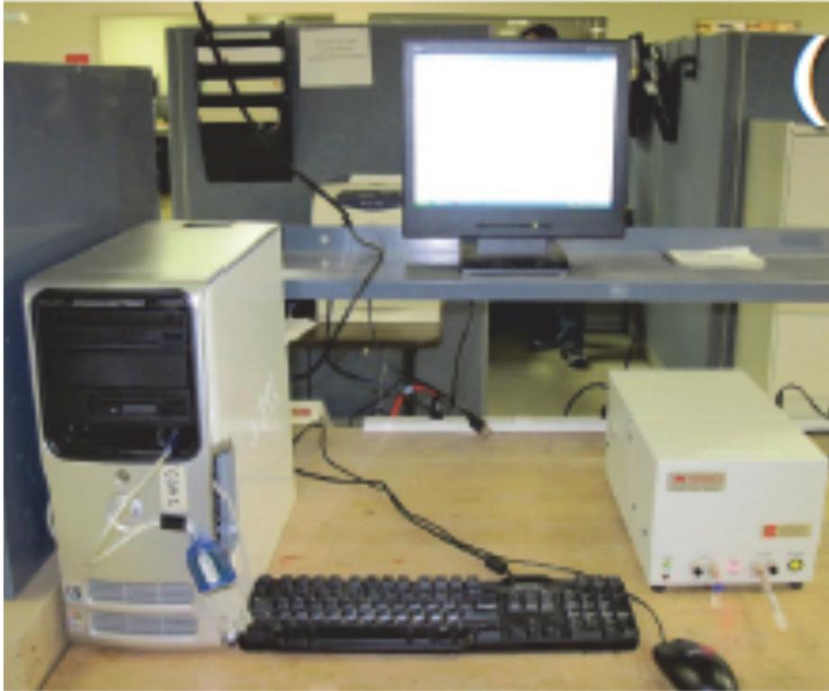
**Figure 3.5. Brookhaven NanoDLS assembly showing DLS unit on the right.**
