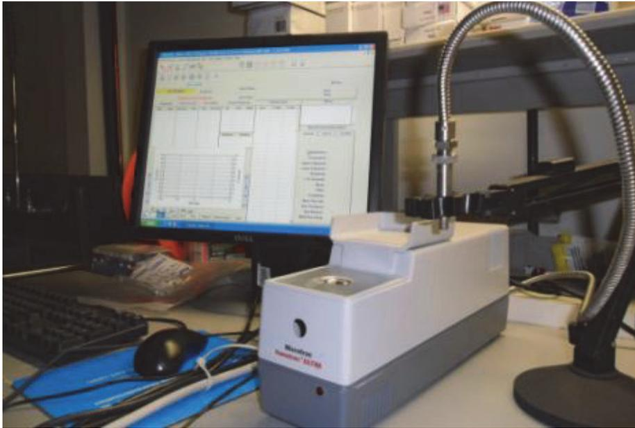
**Figure 3.3. Nanotrak DLS assembly with an independent probe. The probe can also be connected to the sample cell.**
