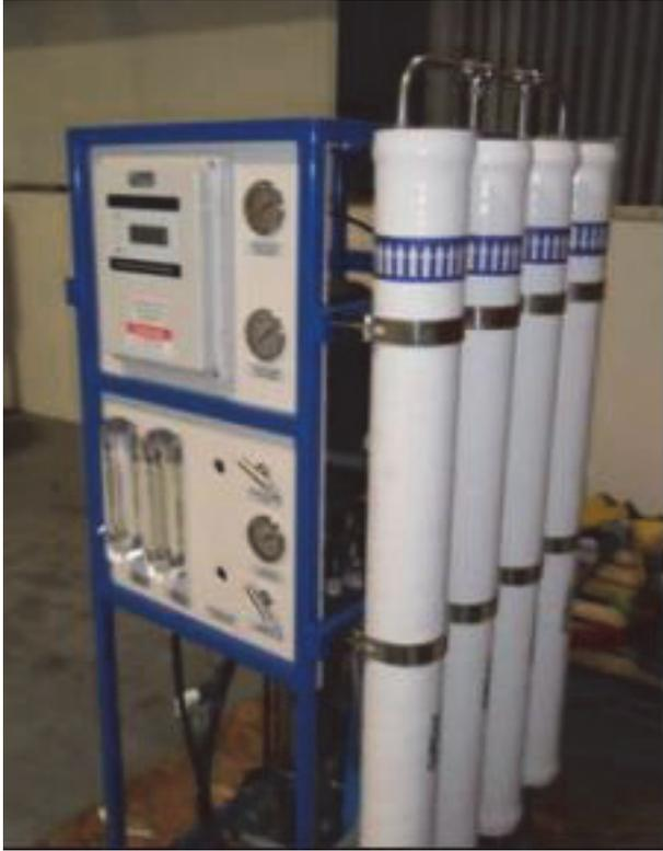
Figure 4.1. RO pilot system used for this study at WRD.
