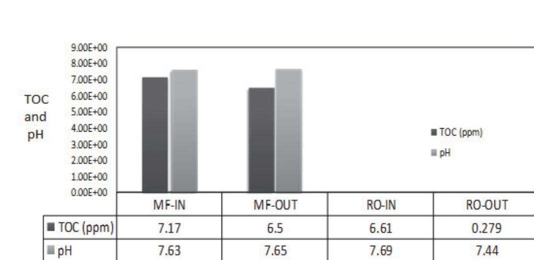
Figure 3.40. Spatial variation in TOC and pH results for RO feed and RO permeate samples.
