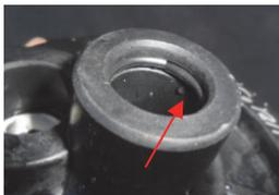
Open O-ring: The O-ring was cut all the way to obtain two separate ends before installing in the groove.
