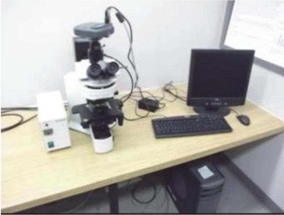
**Figure 3.32. Epifluorescence Microscope (EFM) System.**
