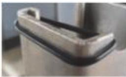
O-ring subjected to stretch. This shape deformation was used to check for any leakage.
