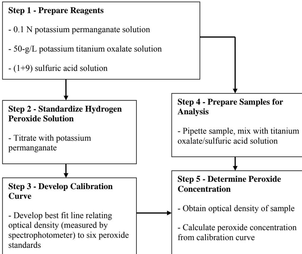
**Figure ES-2. Titanium oxalate method for peroxide detection.**
