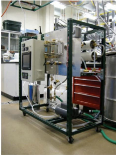
(SCADA) system that downloads operational data including system flow rates, pressure, conductivity, and temperature.
