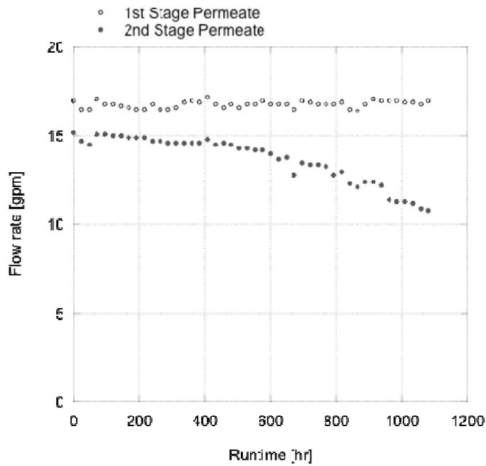
Figure 5.8 First- and second-stage permeate flow rates from vessels in the full-scale system.
