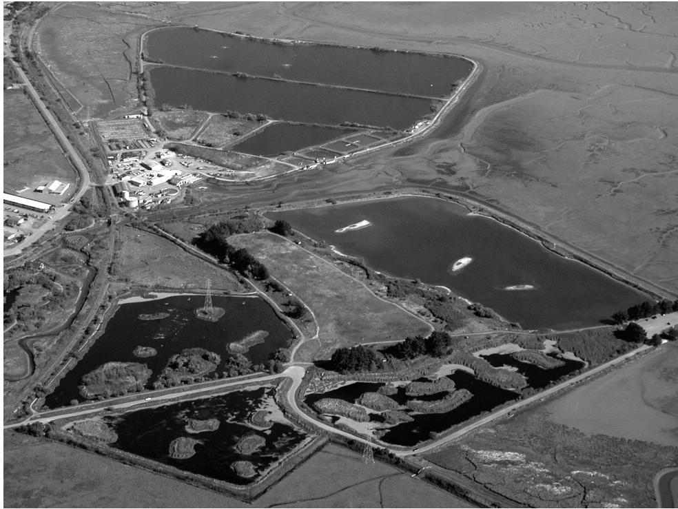
**Figure 3.10. Constructed wetland system for Arcata, CA.**
