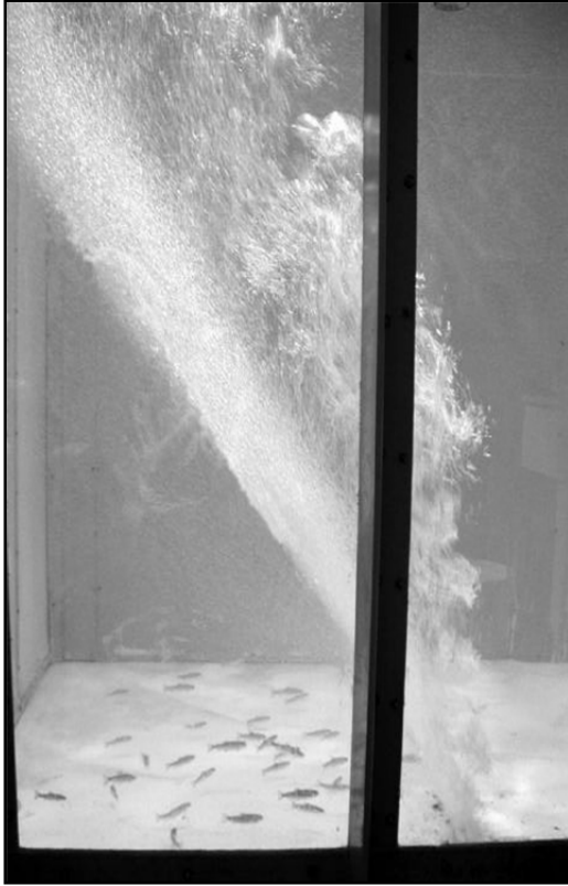
Figure 3.4. Laboratory evaluation of the ability of an air bubble curtain to prevent the movement of fish.
