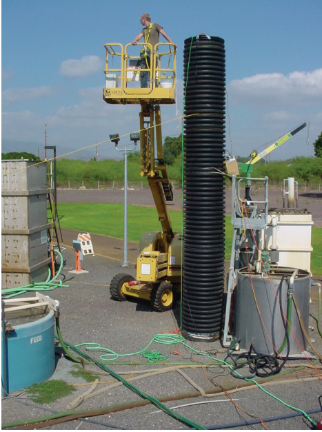
Figure 2.10. Pilot aeration column at MBR pilot test site, Ewa Beach, HI.
