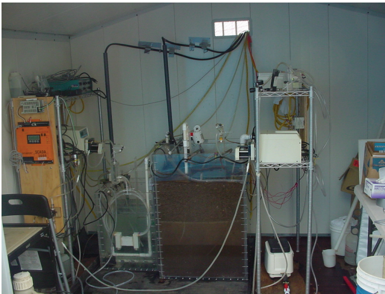
Figure 2.9. Bench-scale Enviroquip (right) and Ionics (left) MBRs at Honouliuli WWTP.
