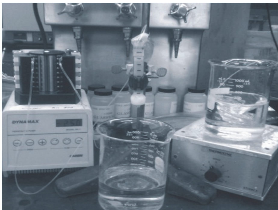
Figure 3.6. Column setup used to evaluate nanomaterials removal.
