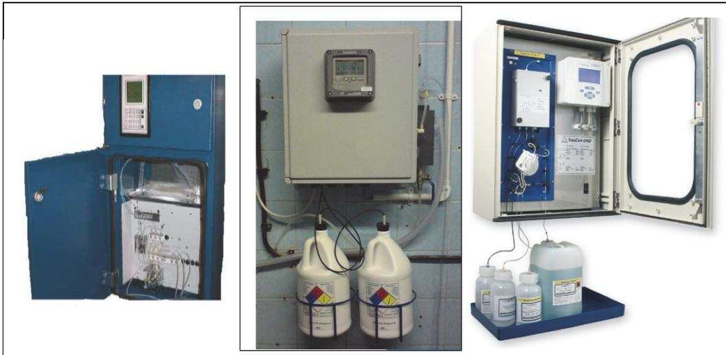
**Figure 2.1. Ammonia analyzers tested during the nitrification reliability study: Waltron, ATI, and TresCon instruments (left to right).**
