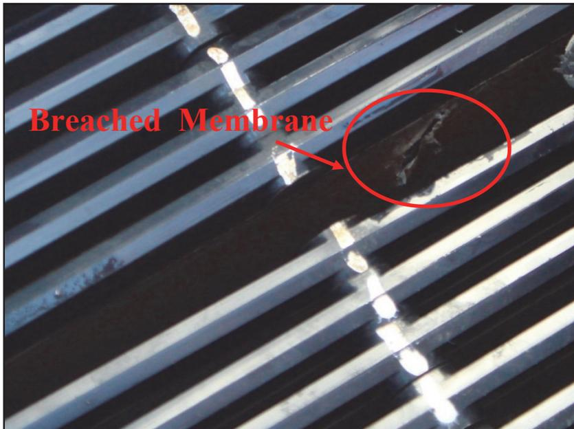
**Figure 6.7. Photograph of the breached membrane.**
