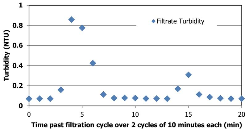
Figure 1.10. Change in filtrate turbidity during membrane breach in MBR.
