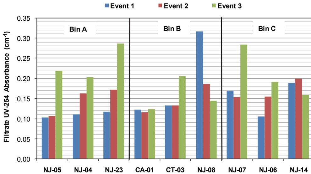
Figure 5.3. Filtrate UV-254 for the selected satellite facilities.
