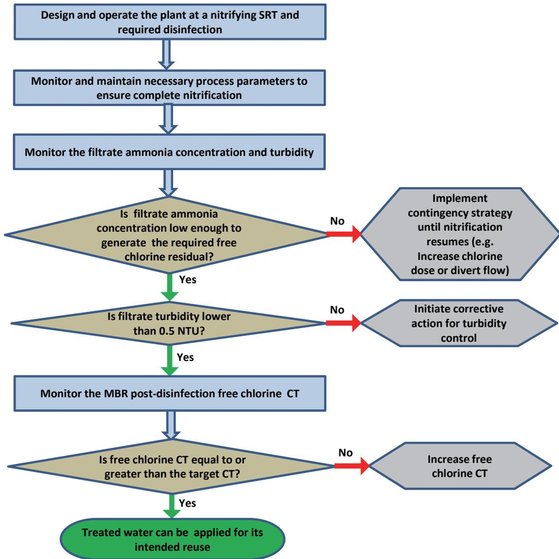
**Figure ES1. Process control strategy for the satellite water recycling facilities to implement lower free chlorine CT values.**
