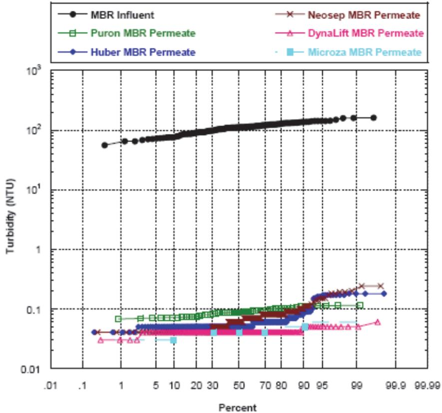
Figure 1.4. Filtrate turbidity for various MBR systems.
