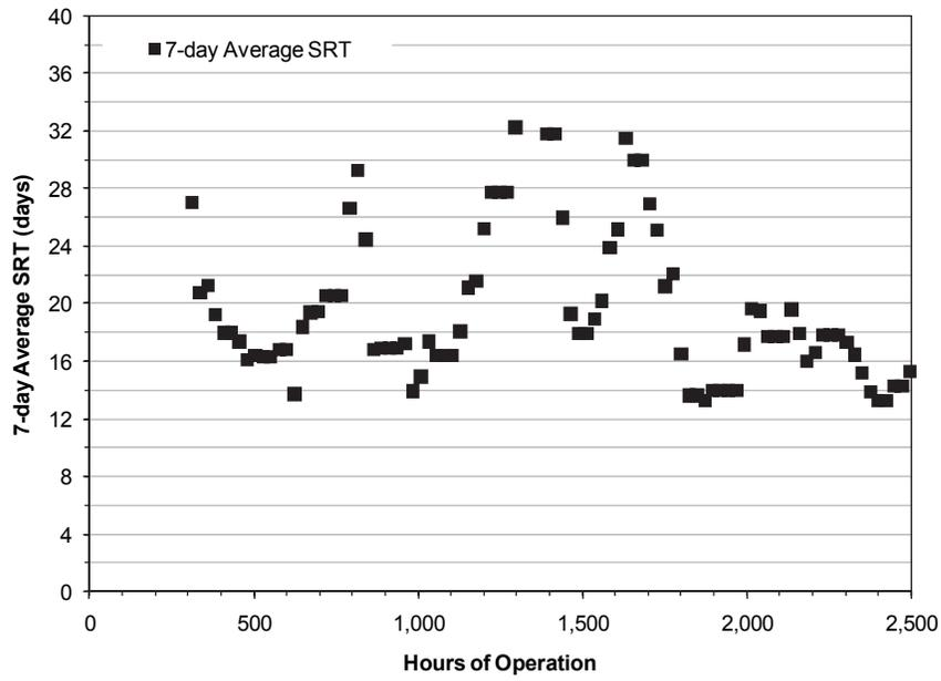
Figure 8.6. Seven-day average SRT at the CA-01 water recycling facility.
