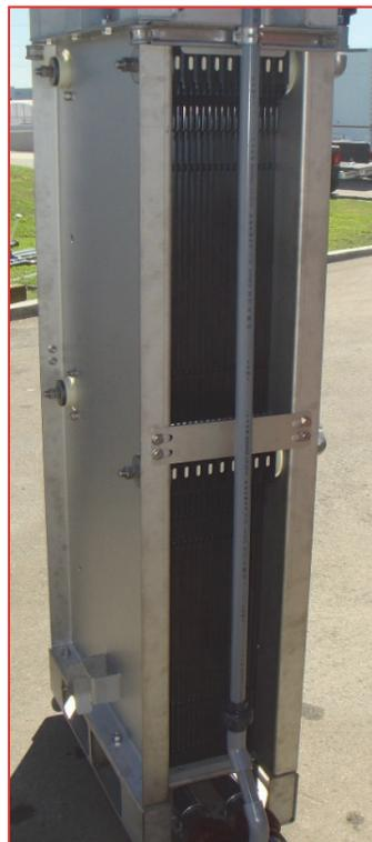
**Figure 3.4. Photograph of the Pilot System A membrane module.**
