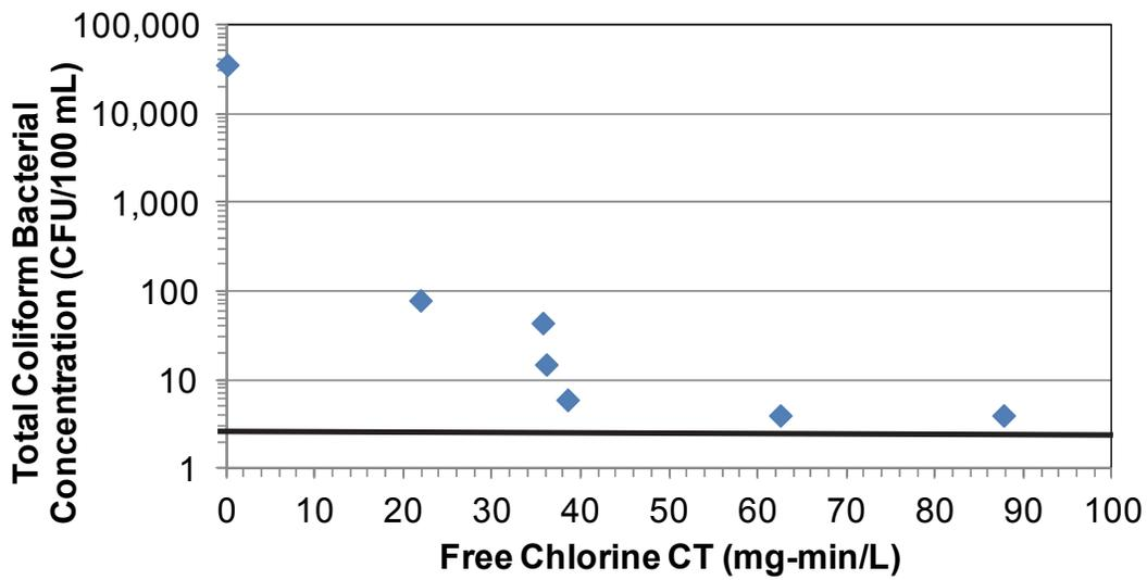
**Figure 7.5. Inactivation of total coliform bacteria and seeded male-specific bacteriophage in MBR filtrate at a turbidity of 6.9 NTU.**
