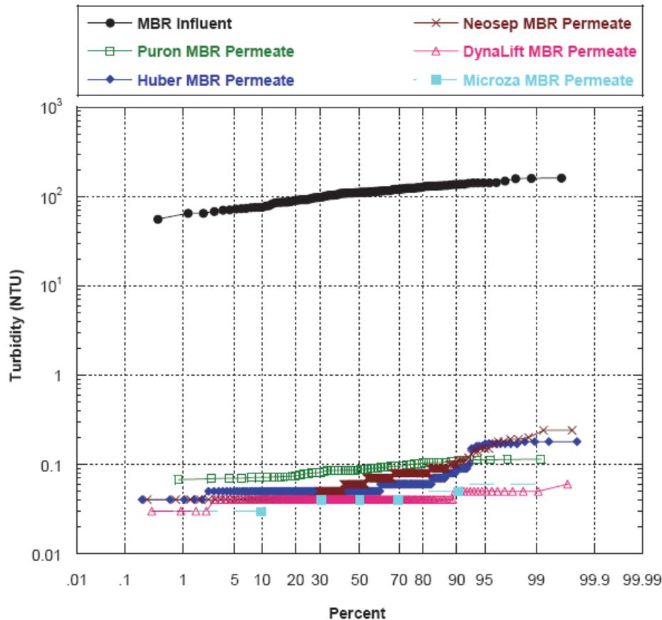
**Figure 1.1. Filtrate turbidity for various MBR systems**
