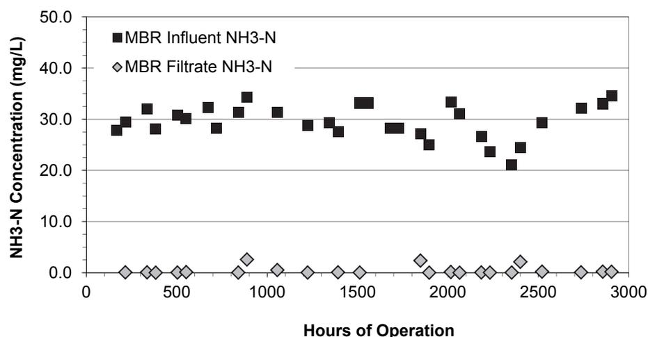
**Figure 1.2. Ammonia removal observed in a submerged MBR system.**
