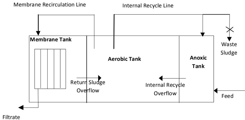
**Figure 3.2. Process schematic of MBR Pilot System A.**
