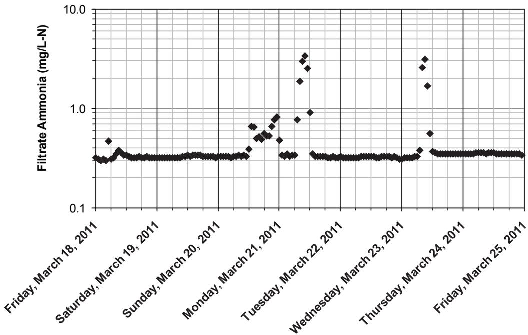
Figure 8.2. Diurnal variations in ammonia concentration in the MBR filtrate at the CA-01 facility measured using an online ammonia analyzer (week of March 18, 2011).
