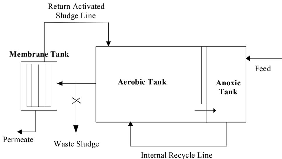
Figure 3.5. Process schematic of MBR Pilot System B.
