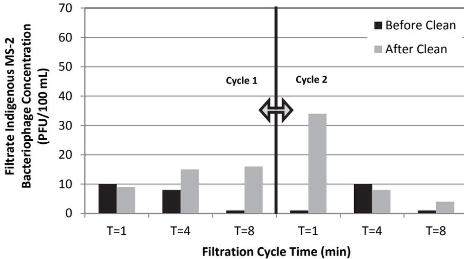
Figure 6.4. Filtrate indigenous male-specific bacteriophage concentrations before and after cleaning the MBR membranes.
