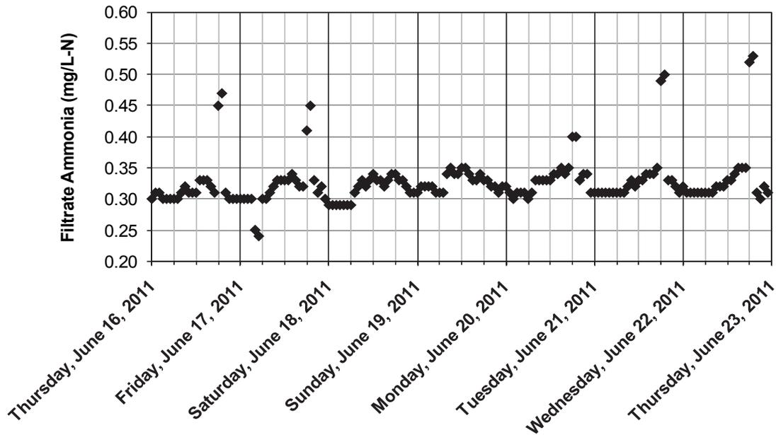
**Figure 8.3. Diurnal variations in ammonia concentration in the MBR filtrate at the CA-01 facility measured using an online ammonia analyzer (week of June 16, 2011).**
