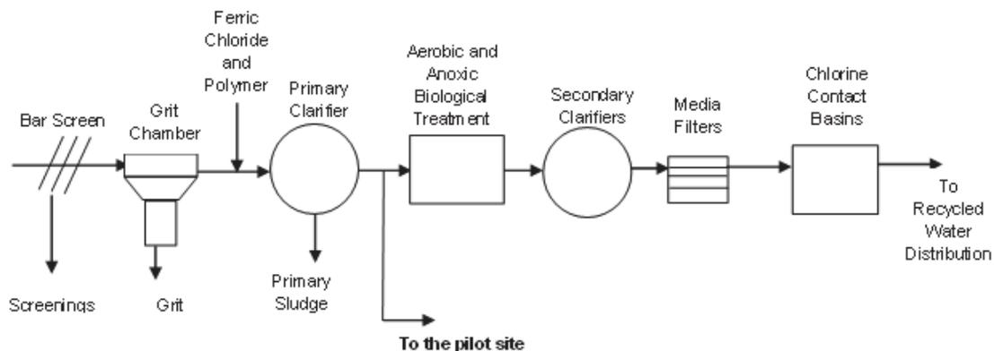
**Figure 3.1. Process flow diagram of the IEUA RP#5.**
