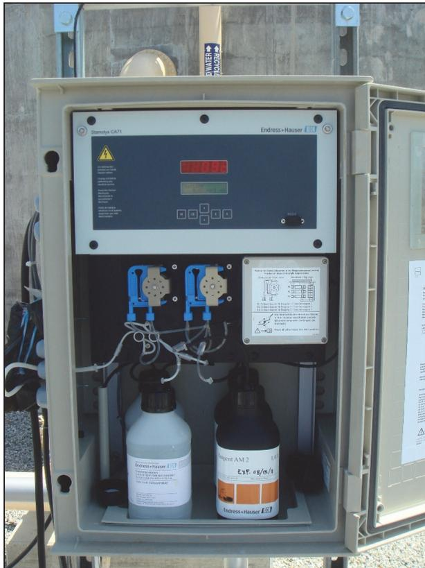
**Figure 3.10. Photographs of the online ammonia analyzer installed at the CA-01 facility.**
