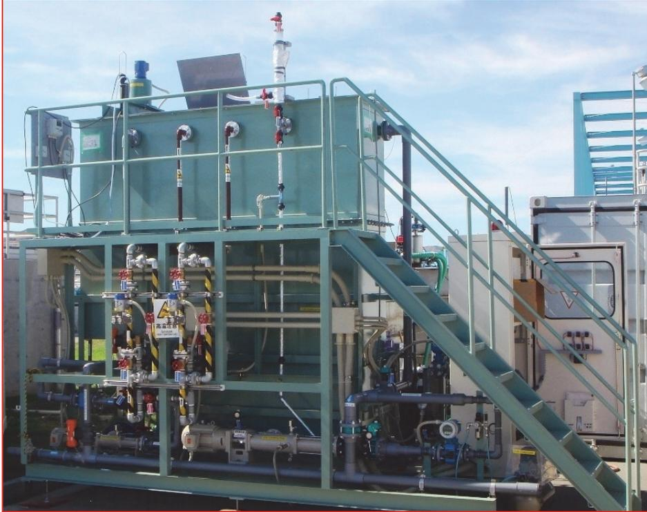
**Figure 3.3. Photograph of MBR Pilot System A.**
