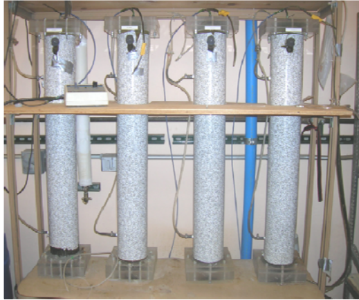
Figure 2.27. Experimental set-up of the PC_{\text{anoxic}} column system.
