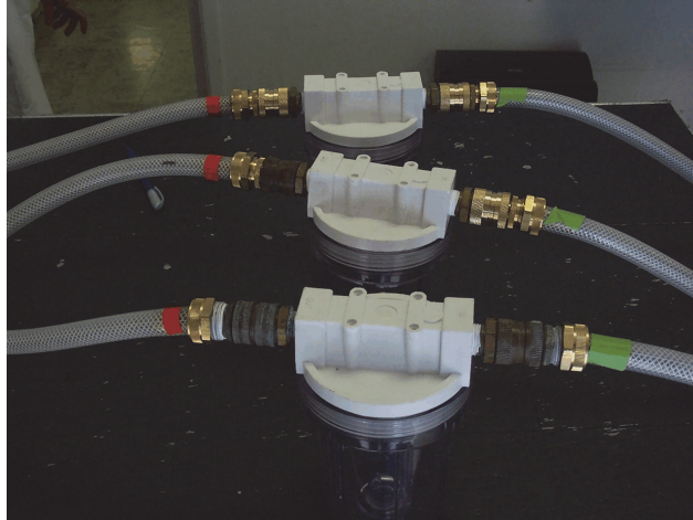
Figure 2. Illustration of the correct influent hose-filter set connections.
