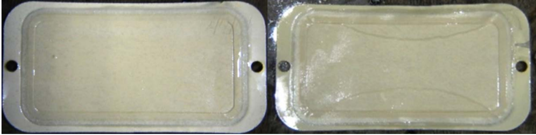
Figure 5.9. RO membrane from the membrane test cell (left: baseline feed test; right: acetate amended feed).
