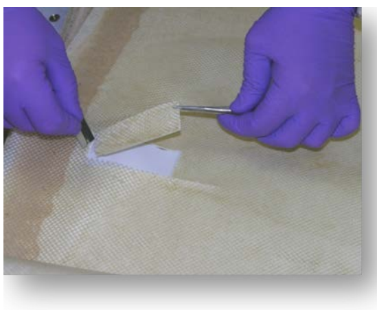
Figure 7.2. Piece of fouled membrane and the spacer material were cut from a sleeve of the Hydranautics ESPA 2 RO element.
