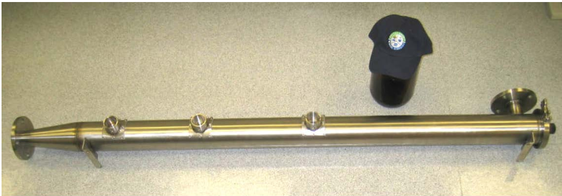
Figure 10.1. Single-lamp reactor with quartz windows for measuring UV intensity of 257-watt LPHO Hg amalgam lamp.
