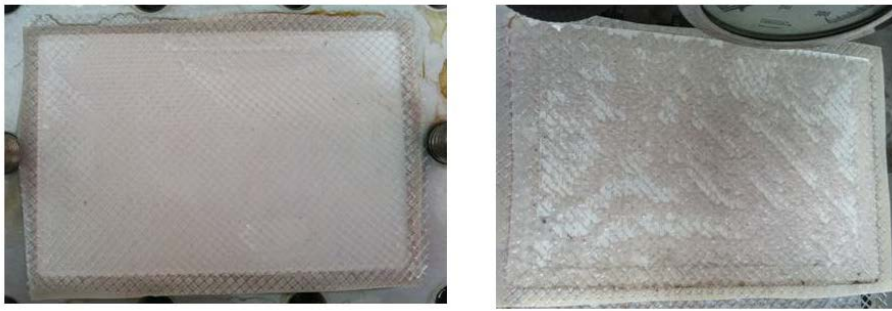
Figure 4.48. Images of fouled ESPA2 control membrane (left) and membrane operated on RO concentrate/brine amended with 30 mg/L of S700 coagulant (right).
