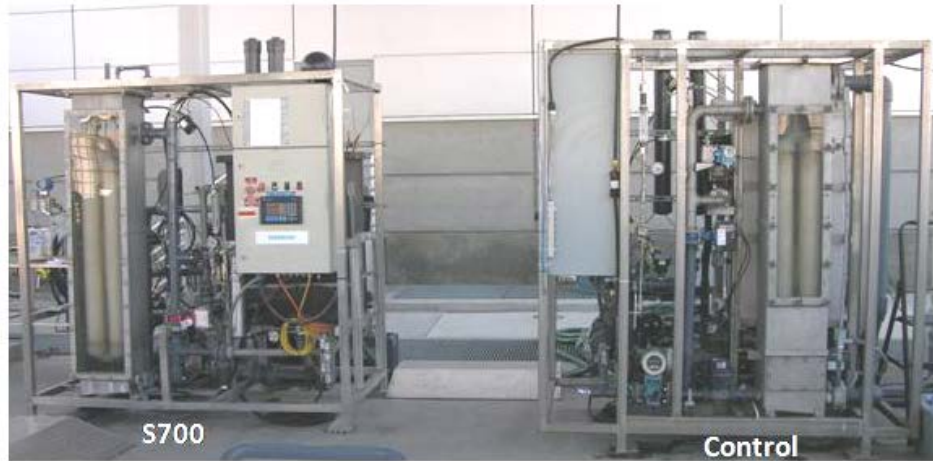
Figure 4.12. Direct filtration 4S10V CS MF pilot units used for MF studies.
